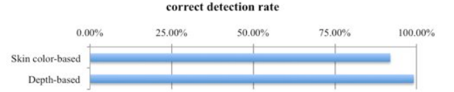
Figure 8: Detection rate on the normal sequence. The color-based detection achieves 92.0% correct detection, while the depth-based detection achieves 99.2% correct detection.
