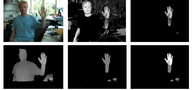
Figure 7: RGB image (top left), depth image (bottom left), skin color probability (top middle), depth image after threshold (bottom middle), skin color probability limited to foreground pixels (top right), and segmented hand (bottom right).
