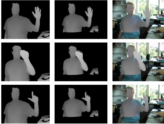
Figure 3: Examples of ToF depth images (left), undistorted and projected to the RGB image coordinates (middle), and overlaid onto the original RGB images (right).
