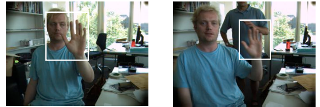
Figure 5: Examples of where the skin color-based hand detection cannot distinguish the hand from the overlapping face or hand in the background.
