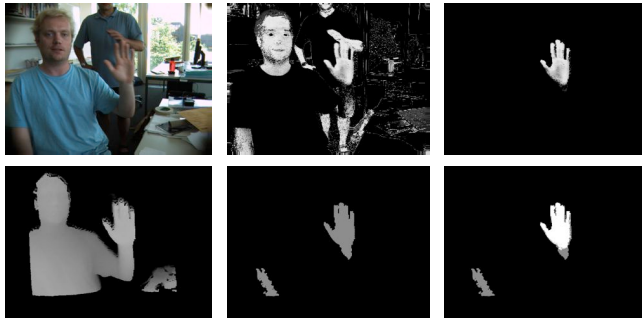
Figure 10: RGB image (top left), depth image (bottom left), skin color probability (top middle), depth image after threshold (bottom middle), skin color probability limited to foreground pixels (top right), and segmented hand (bottom right).
