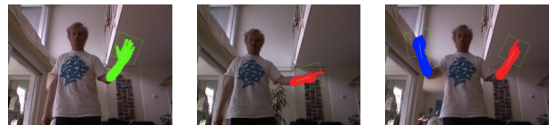
Fig. 5. Examples of the classifier detecting different hand gestures. Green = open hand, red = pointing, blue = fist.
