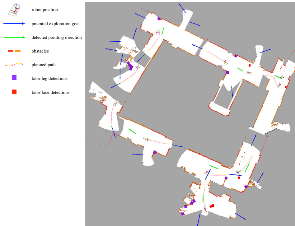
Fig. 9. Detection results of the experiment. The green arrows represent the detected pointing direction after the robot interacted with a human. This pointing direction is then used to select the next exploration goal (blue arrows).
